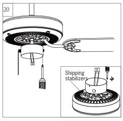
Remove shipping stabilizers from motor assembly.
