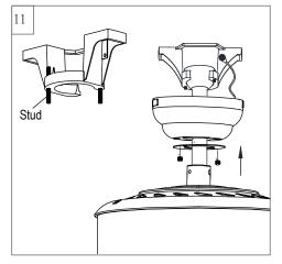
Lift Canopy allowing the 2 studs to protrude through the canopy.
