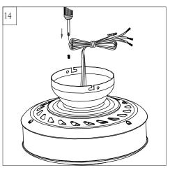
Reinstall the 3 set screws remove in step 12. Tighten screws securely.
