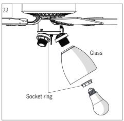
Screw out the socket ring, then push in the glass and lock it with the socket ring.
